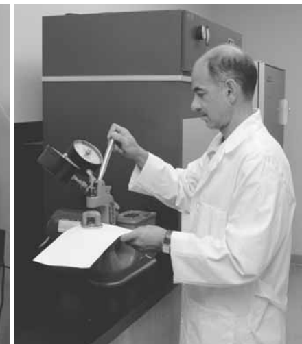
Testing for burst and tensile strength are performed on the B.F. Perkins Mullen® Tester and the Thwing-Albert QC-1000® Materials Tester
